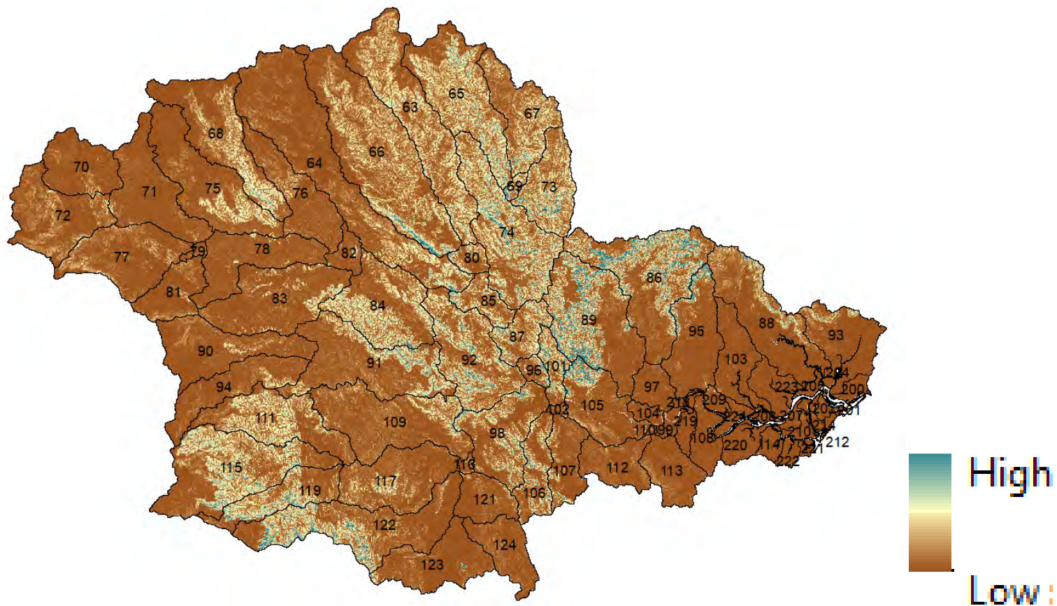
Map A4 - 1 Modelled hillslope erosion in the Manning River catchment (Yang 2019). Likelihood Scores for hillslope erosion were generated from total erosion data for each subcatchment
